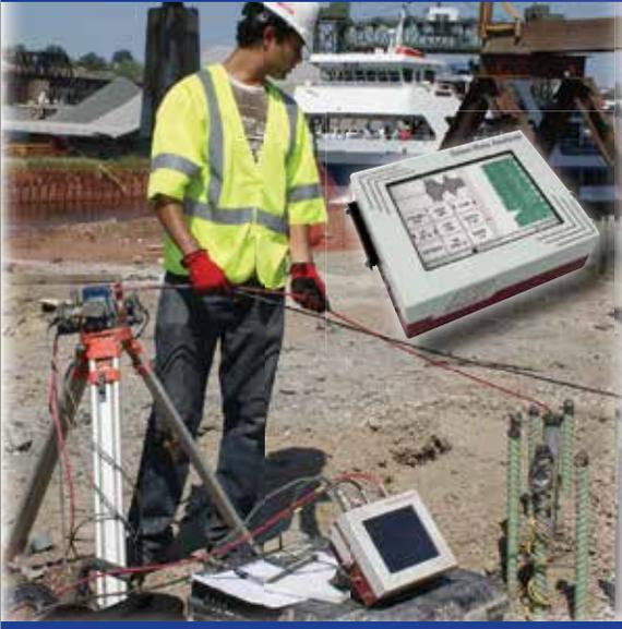
Cross hole sonic logging of drilled shafts per ASTM D6760.
